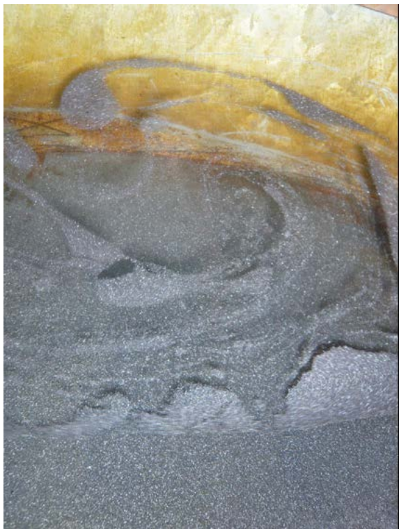
Figure 2. Thick layer of mercury flour floating on water in a pan.
