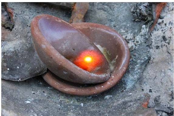
Figure 3. Gold has been smelted out of a heavy mineral concentrate and is ready to be picked out.
