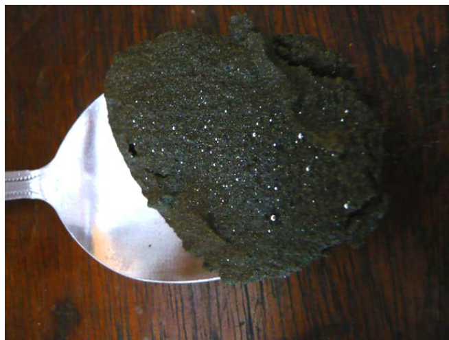
Figure 1. A spoonful of milled gold ore littered with mercury flour.
